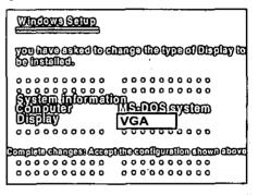
8. Press ENTER key while "Accept the configuration shown above" is highlighted.
